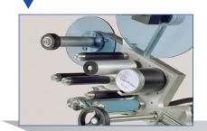
Designed to be extremely versatile the P100 can handle labels up to a maximum of 125mm or 210mm in height and with its rotating label beak is able to apply labels in any plane onto most types of product.
